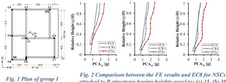
attached to P-structures having heights equal to: (a) 15, (b) 30 and (c) 45 m.
